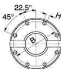
FLANGE WITH FACE KEY - STANDARD TYPE
