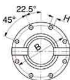
FLANGE WITH FACE KEY - STANDARD TYPE
